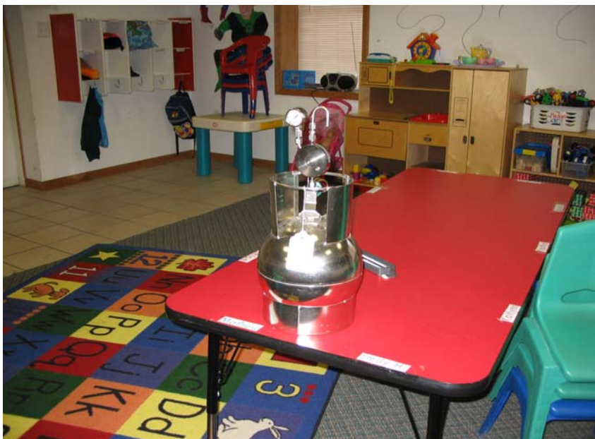
SUMMA ® canister with flow regulator attached and placed at appropriate breathing zone height - ready for sampling.
